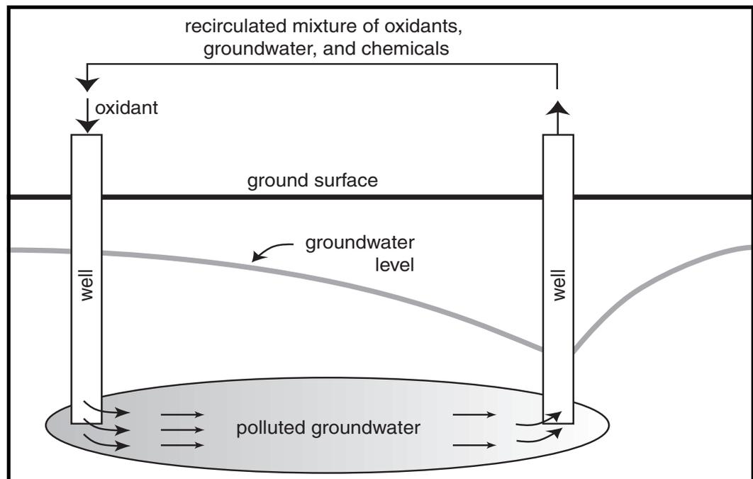
To clean up a site faster, oxidants can be pumped in one well and out another well. This approach helps mix the oxidant with the harmful chemicals in the groundwater and soil. After the mixture is pumped out, it is pumped back (*recirculated*) down the first well. As pumping and mixing continues, more polluted soil and groundwater are cleaned up.
