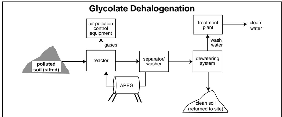
temperature. Once the chemicals evaporate, the cleaned soil can be returned to the site. The gases produced during evaporation are changed into liquids. These liquids are then mixed with other chemicals, such as sodium hydroxide and heated again. A chemical reaction occurs that removes the halogens from some of the chemical and replaces them with hydrogen. This produces a non-toxic salt and a non-toxic chemical. The resulting mixture is then treated using other cleanup methods and recycled.
