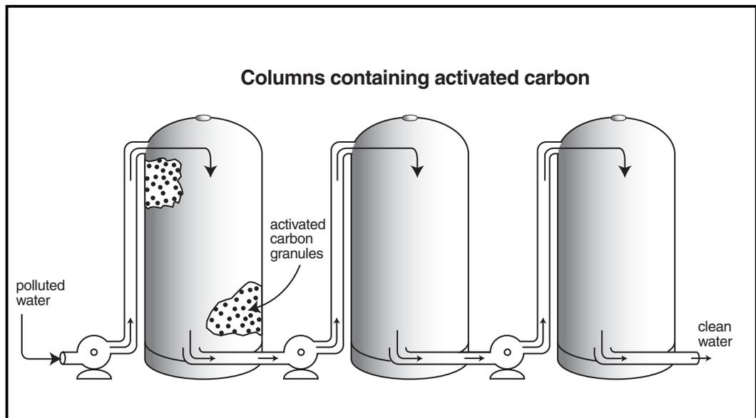
of the granules. The water or air that exits the column is cleaner than the water or air that entered it. If the water or air isn't clean enough, it is pumped into another column or cleaned using another method.
