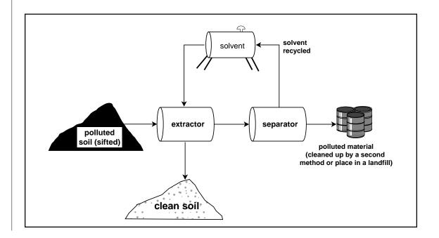
The cleaned soil is tested to make sure that the harmful chemicals have been removed. If harmful chemicals remain, the soil is placed back in the extractor to repeat the process. Clean soil (or sediment) can be placed back on the site.
