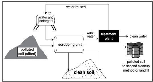
and sometimes detergents, are added to the polluted soil in the scrubbing unit. The mixture of soil and water is passed through sieves, mixing blades, and water sprays. This washes the silt and clay from the larger-grained soil and separates them. Some of the pollution may dissolve in the water or float to the top. The polluted wash water is removed and cleaned up at a treatment plant. The clean water then can be reused in the scrubbing unit or discharged.
