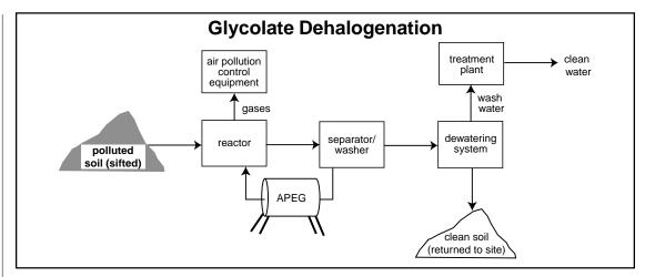
temperature. Once the chemicals evaporate, the cleaned soil can be returned to the site. The gases produced during evaporation are changed into liquids. These liquids are then mixed with other chemicals, such as sodium hydroxide and heated again. A chemical reaction occurs that removes the halogens from some of the chemical and replaces them with hydrogen. This produces a nontoxic salt and a non-toxic chemical. The resulting mixture is then treated using other cleanup methods and recycled.
